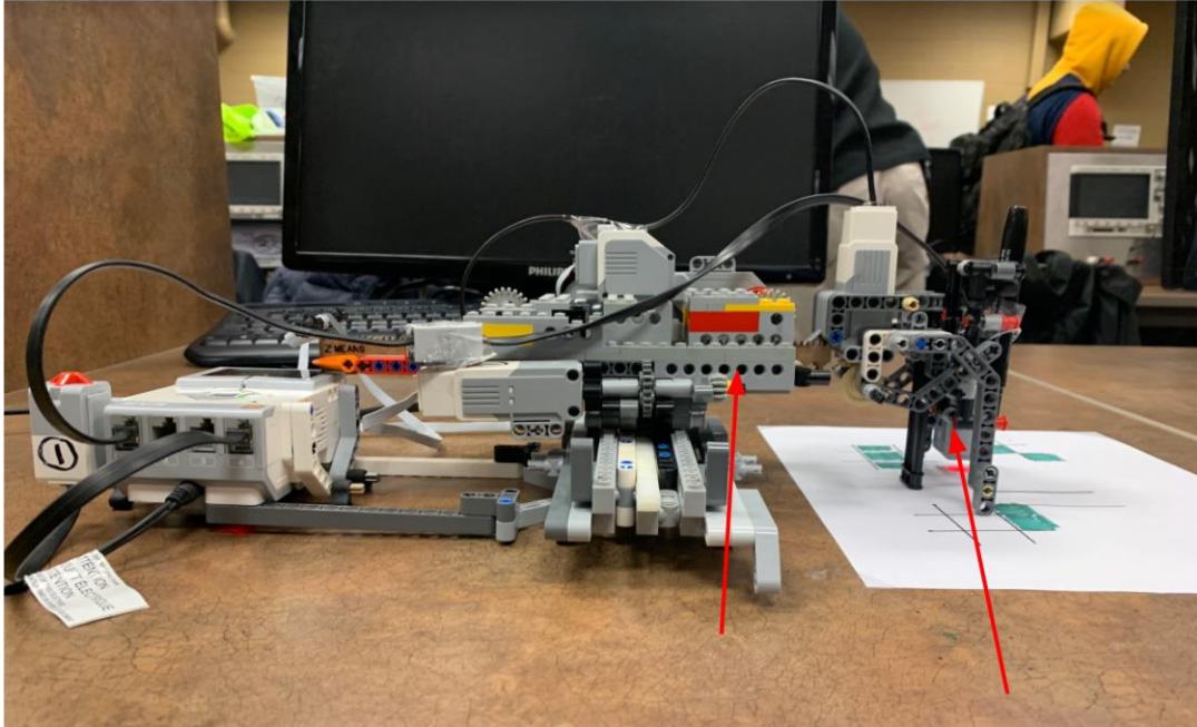
Figure 8. Central Housing (Left) and Extension Arm (Right).
